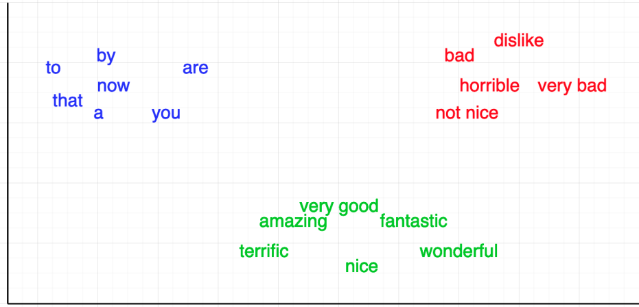
Figure 3.2: A two-dimensional (t-SNE) projection of word embeddings. Adapted from [26] and [21]
